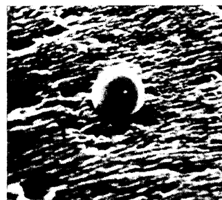
Figure 5. Isometric diamond crystal grown on a (111) face, photographed in a scanning electron microscope. Crystal diameter 20 \mu\text{m} .
